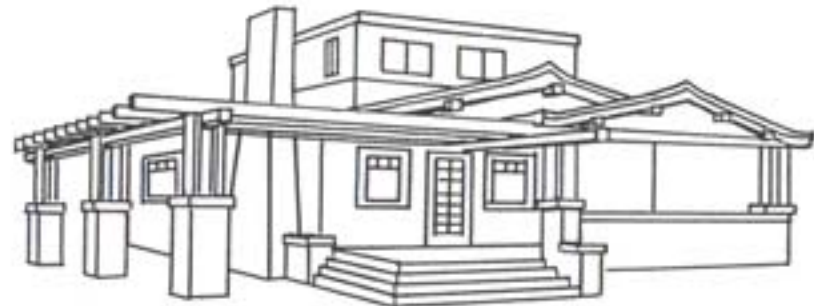
Flat roofed, unarticulated addition is not acceptable with Craftsman style
