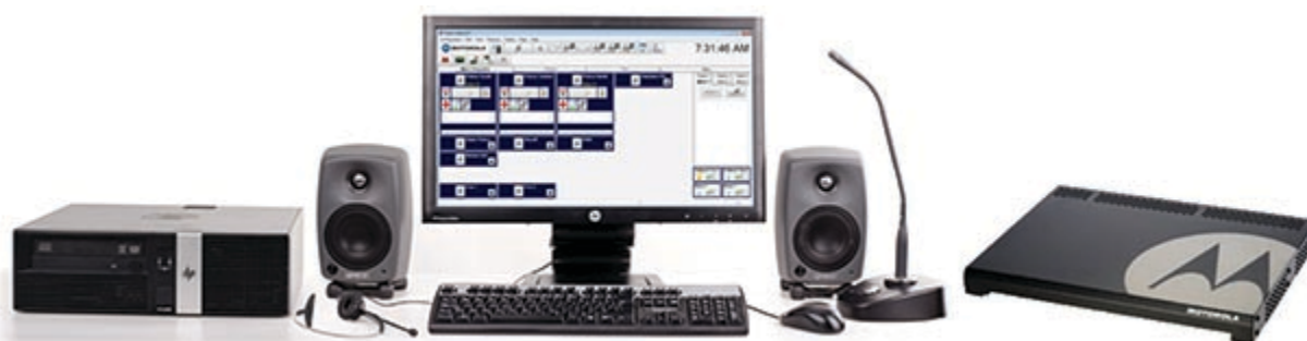
Figure 1: MCC 7500 Dispatch Console. The Console includes desktop PC, headset, speakers, display, keyboard, mouse, microphone, and Voice Processor Module
