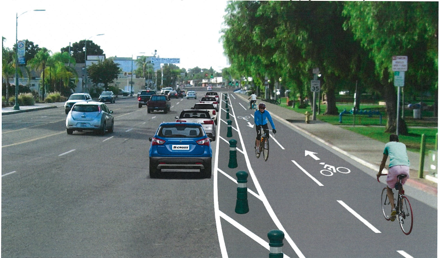
Figure 2: Photo Simulation of the Proposed Class IV Bikeway (Cycle Tracks) on N. Broadway
