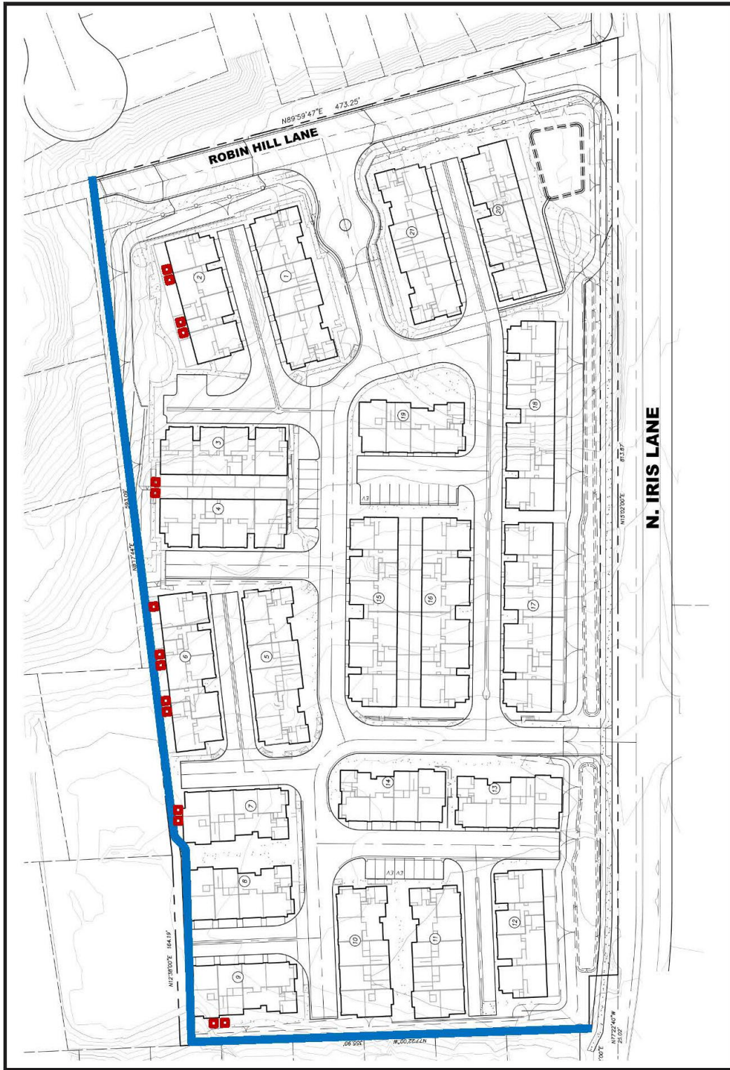
Figure 3.11-2. Locations of Proposed HVAC Units
