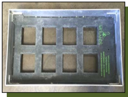
Refilling tray for media replacement.
