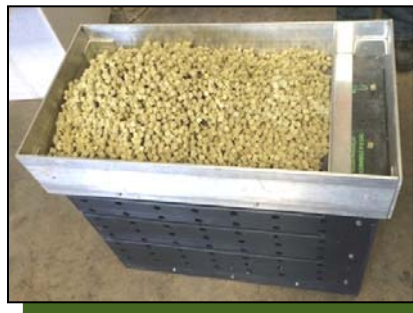
Refilling tray on cartridge with bulk media.
