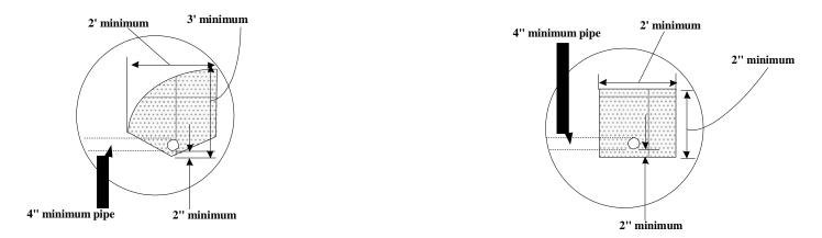
Filter Material: Minimum of 5 ft<sup>3</sup>/linear foot of pipe or 4 ft<sup>3</sup>/linear foot of pipe when placed in square cut trench.
